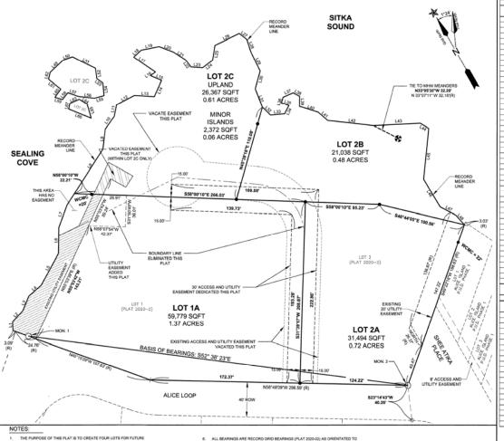
ALL BEARINGS ARE RECORD GRID BEARINGS (PLAT 2020-02) AS ORIENTATED TO THE BASIS OF BEARINGS, OBSERVED THIS SURVEY, DISTANCES SHOWN ARE REDUCED TO HORIZONTAL EIELD DISTANCES
