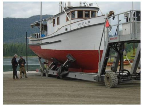
unnecessarily without additional planning and market knowledge. Phase 1 would provide haul out and Uplands maintenance space to the vast majority of the local fleet, excluding only the larger seiners and tenders. The use of a hydraulic trailer is an excellent first step to an efficient haul out service. Most yards use either a trailer alone or in conjunction with a travel lift. Some advantages of hydraulic trailers, either in general or in the case of the Park, are:
