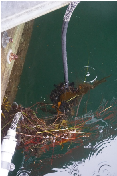
Photograph 20: Cable weighted by encrusted marine life.
