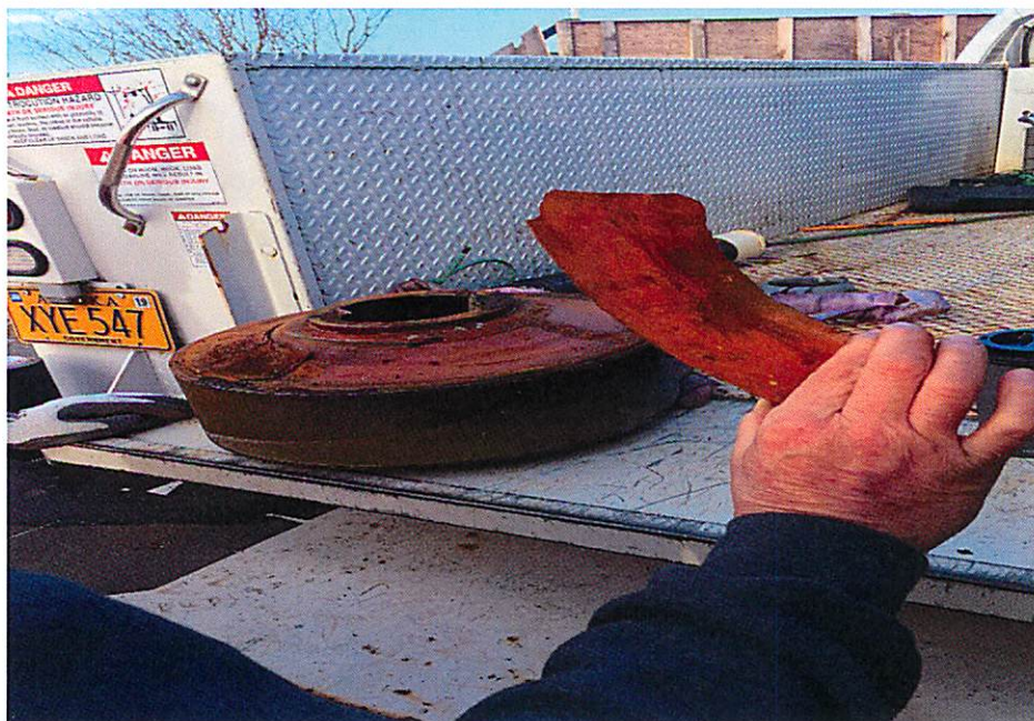
Impeller and piece of volute
