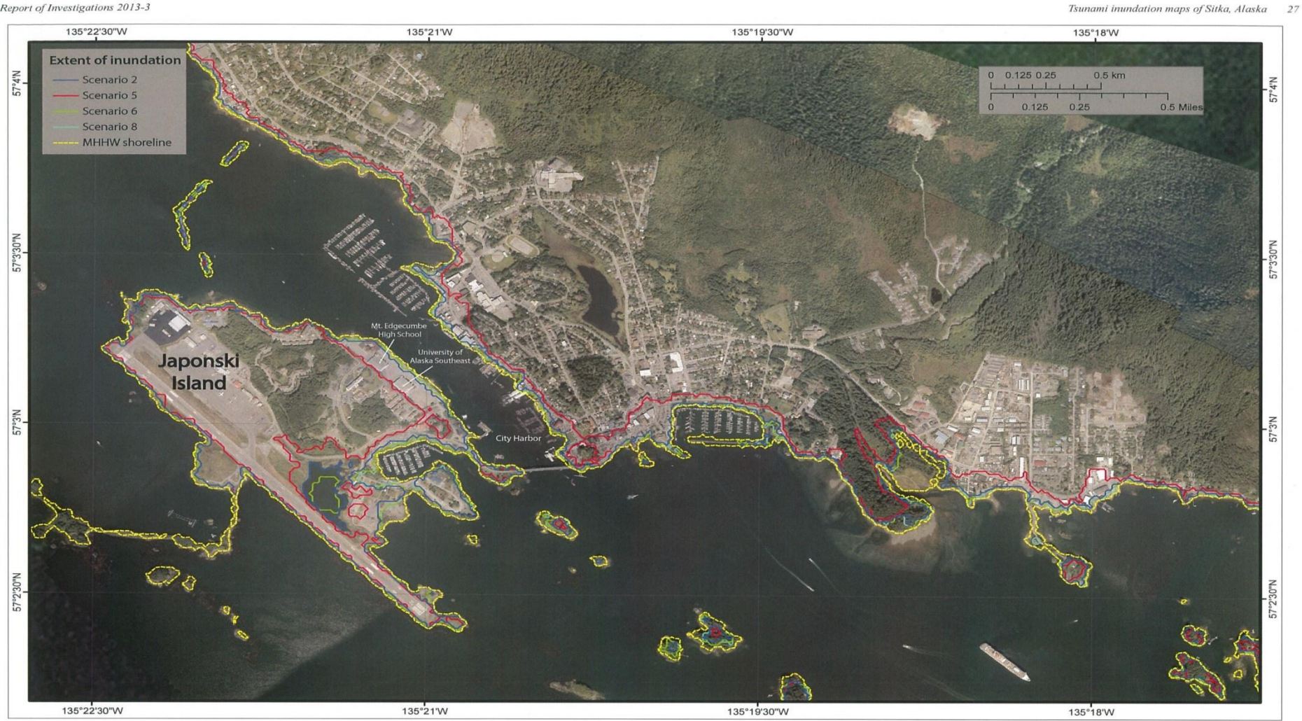
Figure 16. Calculated potential inundation in Sitka for Scenarios 2, 5, 6, and 8 with respect to the MHHW shoreline.
