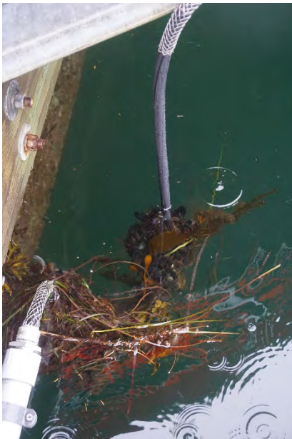
Photograph 20: Cable weighted by encrusted marine life.
