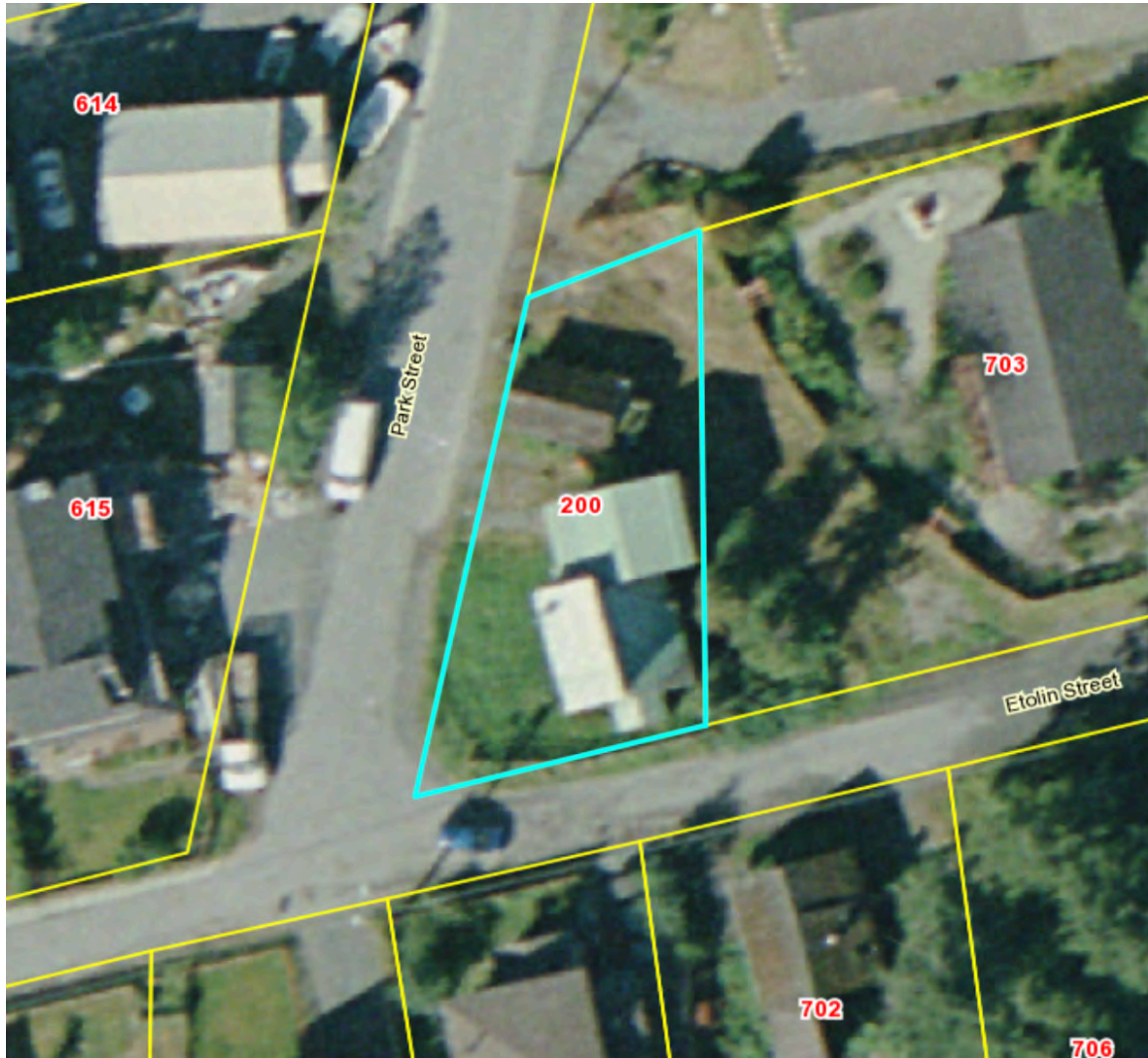
Figure 1. 200 Park Street. As you can see, our property line is setback from the paved portion of Park (drawings from City of Sitka from the stormwater/sewer project in 2007 show about 8'-10' between pavement and the property line). The area just to the east is a triangular easement that belongs to 703 Etolin.
