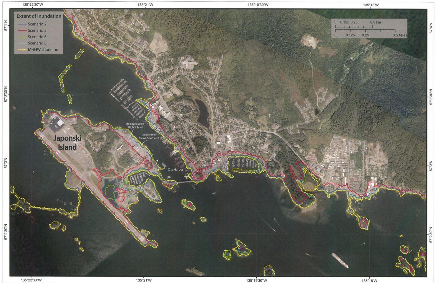
Figure 16. Calculated potential inundation in Sitka for Scenarios 2, 5, 6, and 8 with respect to the MHHW shoreline.
