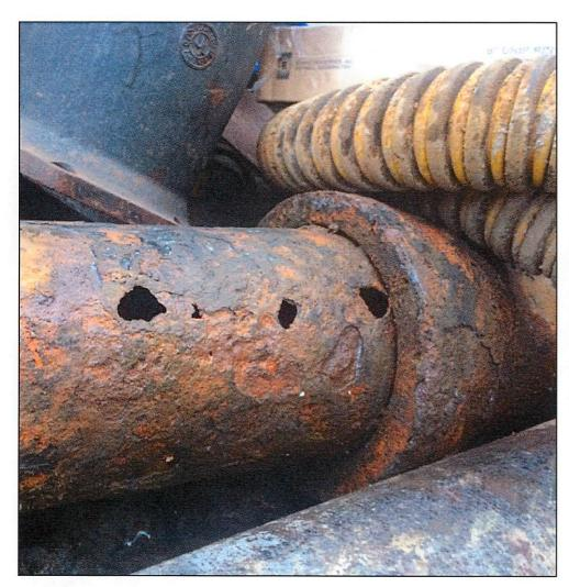
A portion of the Landfill Lift Station force main, shown above, was removed after leaks developed in 2015. The leaks were due to the corrosive leachate pumped by the lift station. The lift stations improvement project will replace the ductile iron pipe with a pipe less vulnerable to corrosion.
