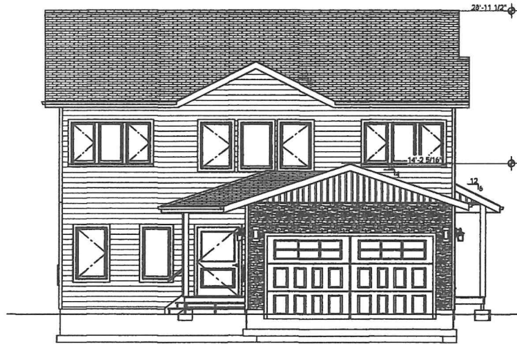
Exterior Elevation Left 1/8" = 1 ft
