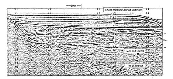
For this investigation the data will be acquired with a medium frequency (350 to 800 Hz) seismic reflection system to map the depth to bedrock or acoustic basement to approximately 100 to 150 feet
