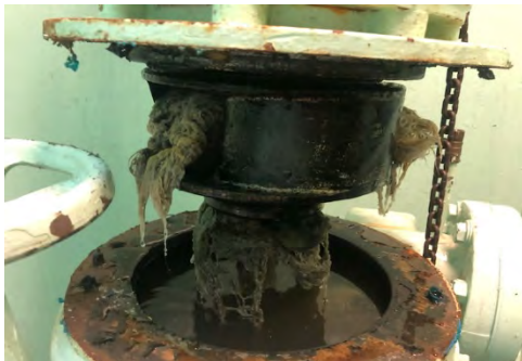
This photo shows the impeller bound with wipes
